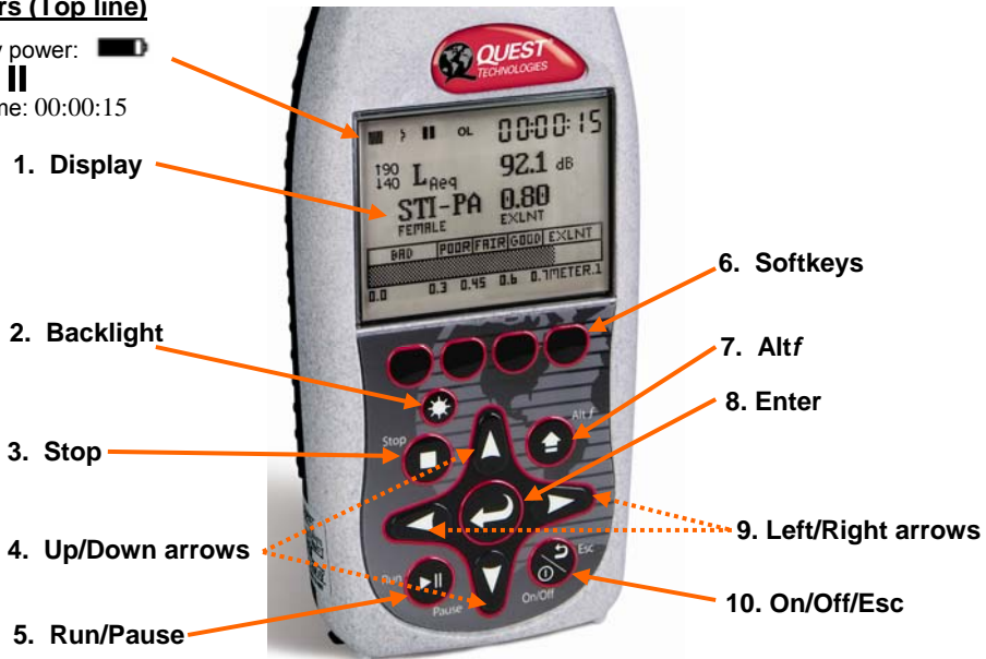
Figure 2-3: Verifier keypad and display explained
