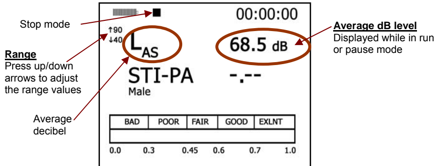
Figure 5-1: Level set-up and average decibel level
