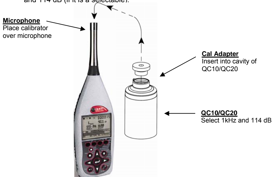
Figure 4-1: Attaching calibrator to the Verifier
