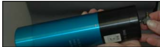
Figure 1-1: Attaching accelerometer to calibrator
